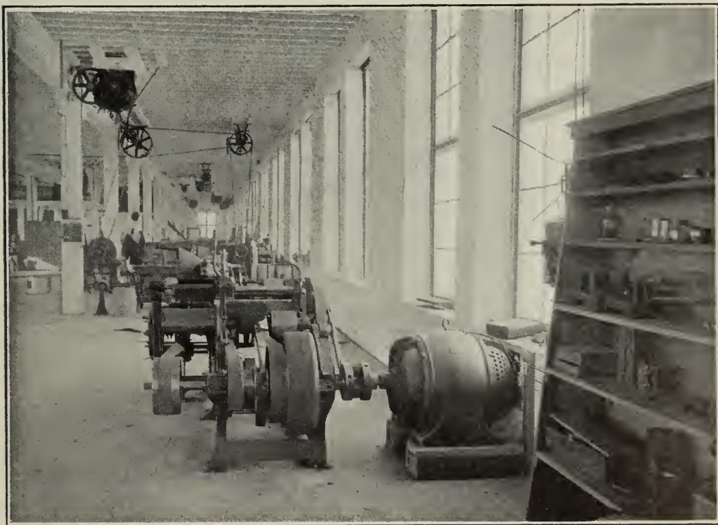
JOINTING MACHINE IN A WOOD-WORKING FACTORY, DIRECT-DRIVEN THROUGH A COUPLING BY TRIUMPH ELECTRIC COMPANY'S MOTOR.
